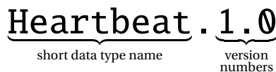
Figure 3.5: Reference to an external composite data type definition located in the same namespace
